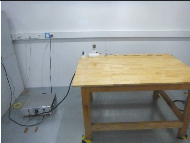
Conducted Emissions Test Setup Front View
