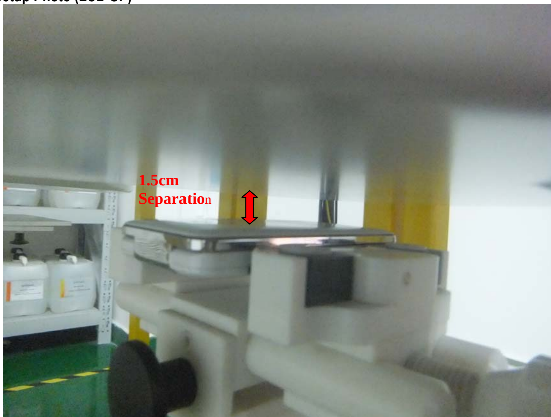
Body Setup Photo (LCD DOWN)
