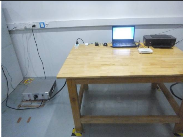
Conducted Emissions Test Setup – Front View
