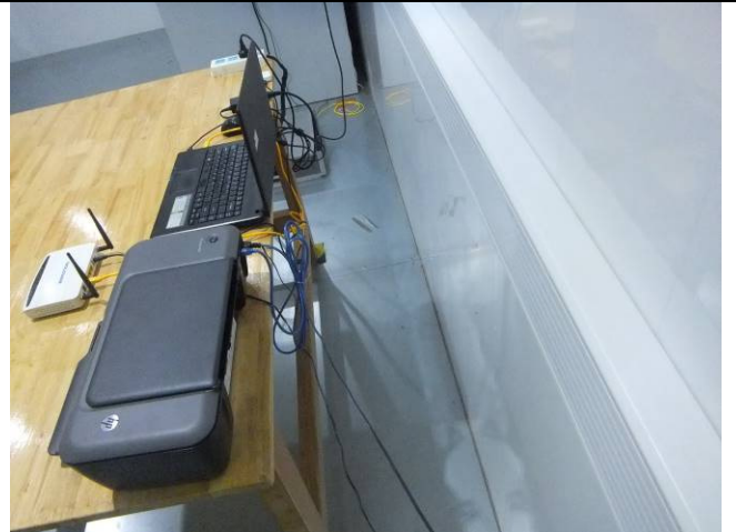
Conducted Emissions Test Setup – Side View
