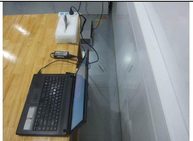
Conducted Emissions Test Setup – Side View
