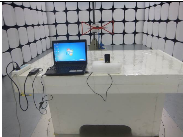
Conducted Emissions Test Setup – Front View
