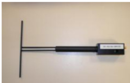
Figure 1 – Satimo COMOSAR Validation Dipole
