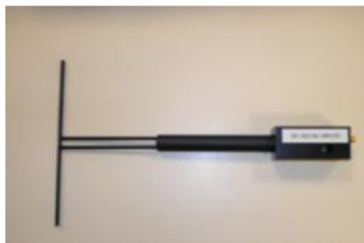
Figure 1 – Satimo COMOSAR Validation Dipole
