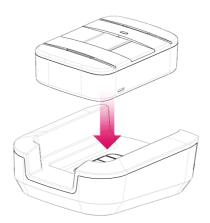
2. Lower your "R3 Medical Alert Device" into the Charging Cradle until the Charging Contacts on both the "R3 Medical Alert Device" and Charging Cradle make contact. You will hear a tone from the Speaker indicating that the device is placed properly and charging.
