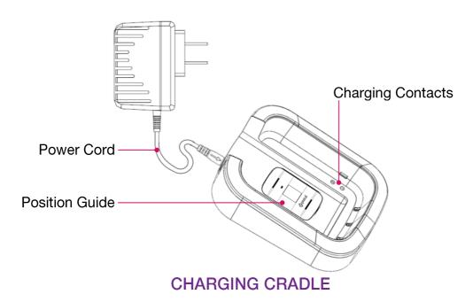
Power Cord – Provides power to the Charging Cradle from a wall outlet.
