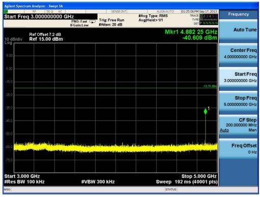
Test Plots (GFSK) - 5 GHz - 7 GHz (RBW:100 kHz, VBW: 300 kHz) Spurious Emission (Mid-CH)
