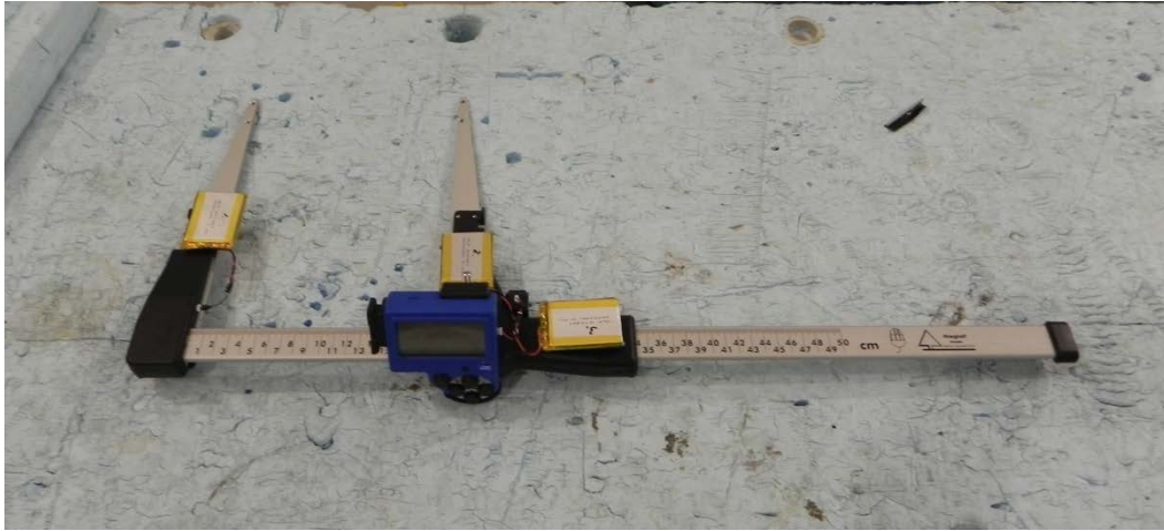
EUT with all three transceivers and external large capacity batteries.
