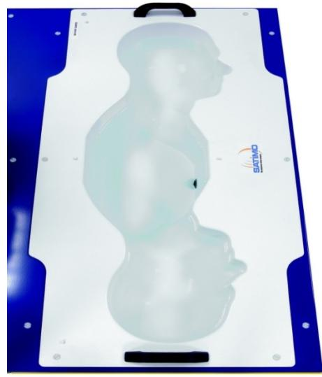
The bottom plate contains three pairs of bolts for locking the device holder. The device holder positions are adjusted to the standard measurement positions in the three sections. A white cover is provided to tap the phantom during off-periods to prevent water evaporation and changes in the liquid parameters. On the phantom top, three reference markers are provided to identify the phantom position with respect to the robot.
