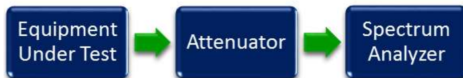
Figure 4. Occupied Bandwidth Test Setup
