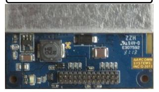
The Aarcomm model RM1-900MRTR is a frequency hopped spread spectrum (FHSS) transceiver module designed to be compatible with U.S. (FCC Part 15.247) and Canadian (RSS-210) regulations for license free use in the 902-928MHz ISM band.
