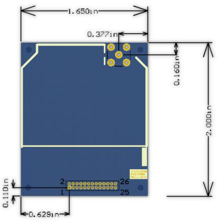
This information should be referenced when designing the host interface PCB to the RM1-900MRTR
