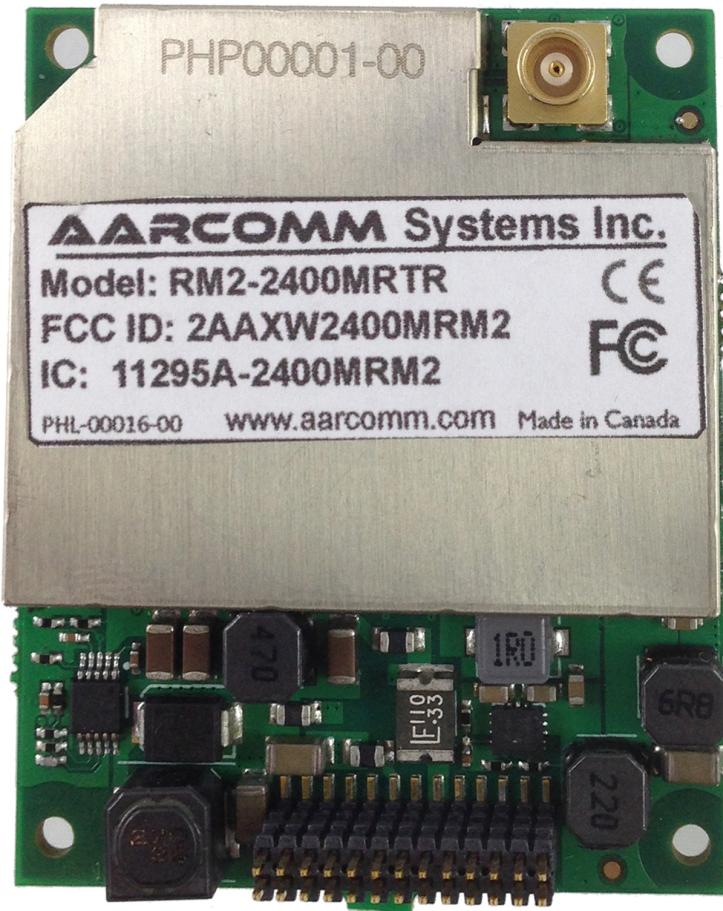
The Aarcomm model RM2-2400 MRTR is a frequency hopped spread spectrum (FHSS) transceiver module designed to be compatible with U.S. (FCC Part 15.247), Canadian (RSS-210) and European (EN 300-328) regulations for license free use in the 2.4-2.483 GHz ISM band.
