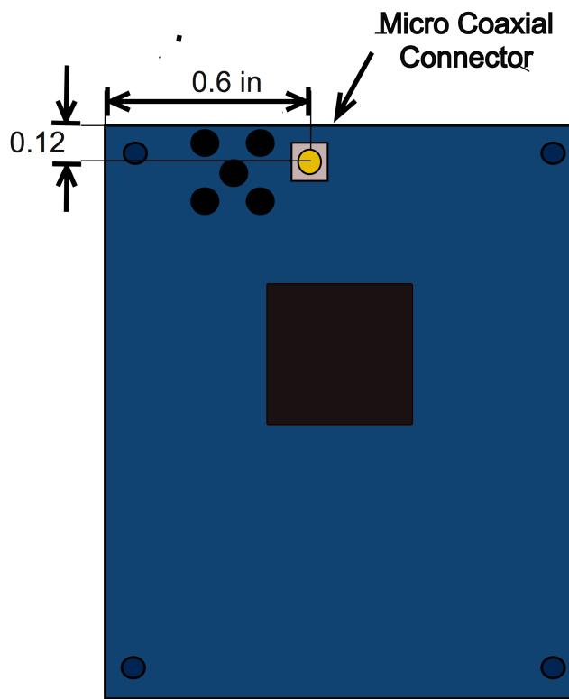
This information should be referenced when designing the host interface PCB to the RM2-2400MRTR
