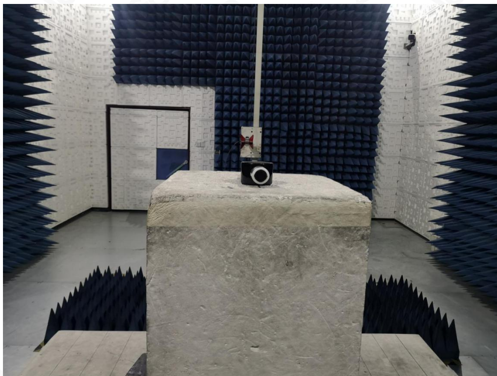
RADIATED EMISSION TEST SETUP ABOVE 1GHZ
