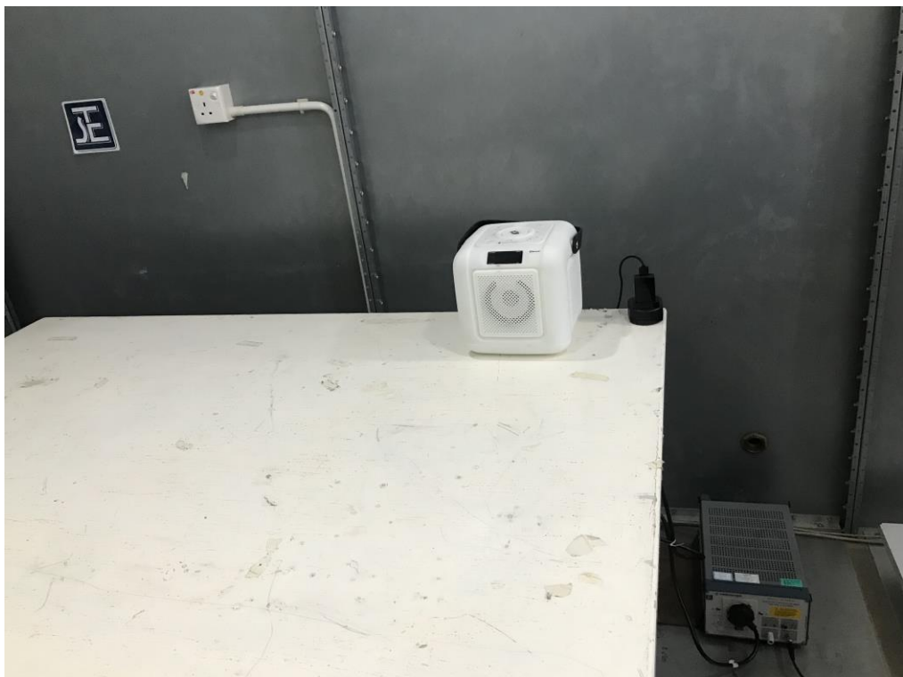
Measurement of Conducted Emission Test Set Up
