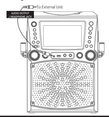
Connect an external device by using an appropriate cable (3.5mm audio cable not included) as shown.
