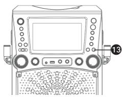
AUTO VOICE CONTROL can be activated by pressing the AUTO VOICE CONTROL ON/OFF button. The vocals on a multiplex recording will be muted as soon as the singer begins singing into the microphone. When the singer stops singing, the recorded vocals on the multiplex recording will resume to normal.
