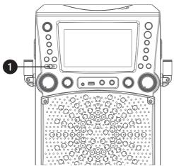
To illuminate the disco light and get your desired lighting effect, slide the **Disco Light DIMMER** slide switch from the MIN position to your desired level.
