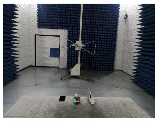
RADIATED EMISSION TEST SETUP ABOVE 1GHZ
