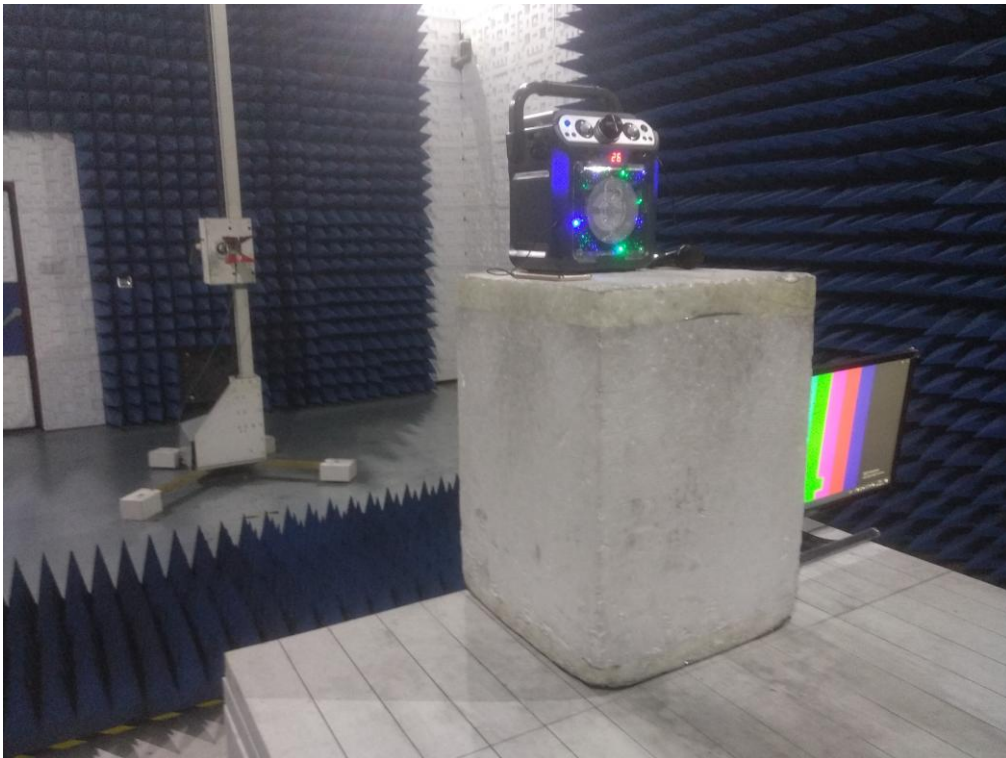
RADIATED EMISSION TEST SETUP ABOVE 1GHZ
