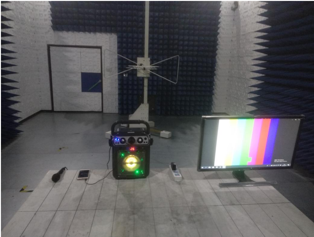
RADIATED EMISSION TEST SETUP ABOVE 1GHZ
