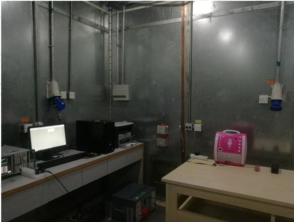
FCC RADIATED EMISSION TEST SETUP
