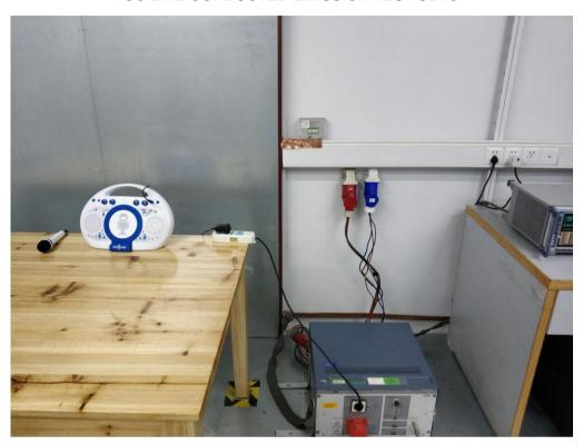
FCC RADIATED EMISSION TEST SETUP
