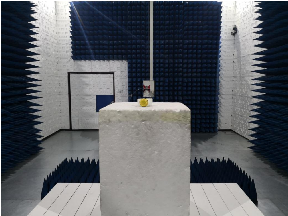
RADIATED EMISSION TEST SETUP ABOVE 1GHZ
