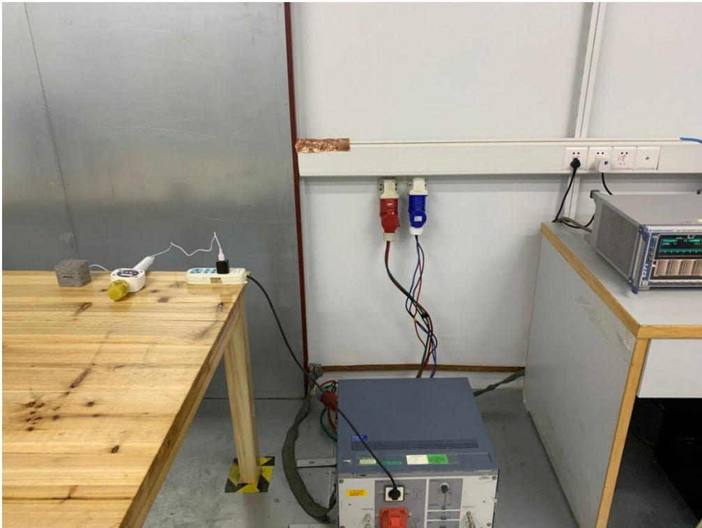
CONDUCTED EMISSION TEST SETUP
