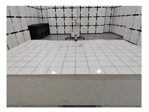
Set-up for Radiated Spurious Emission, Above 1GHz
