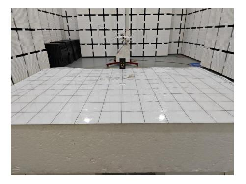
Set-up for Radiated Spurious Emission, Below 1GHz
