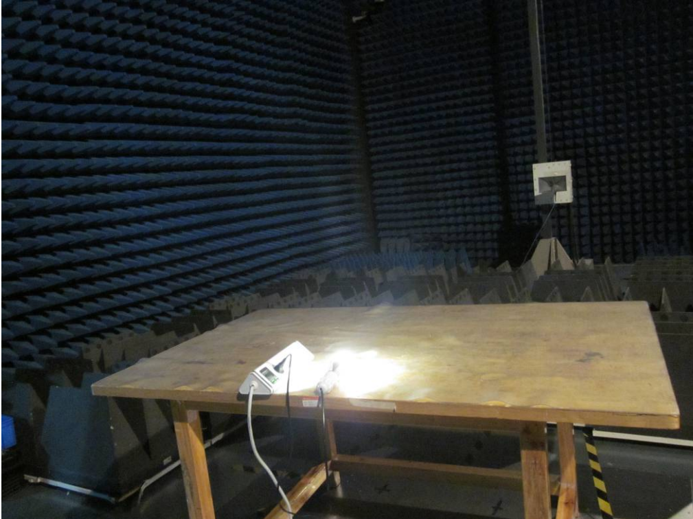
17.2 Photograph – Conducted Emission Test Setup
