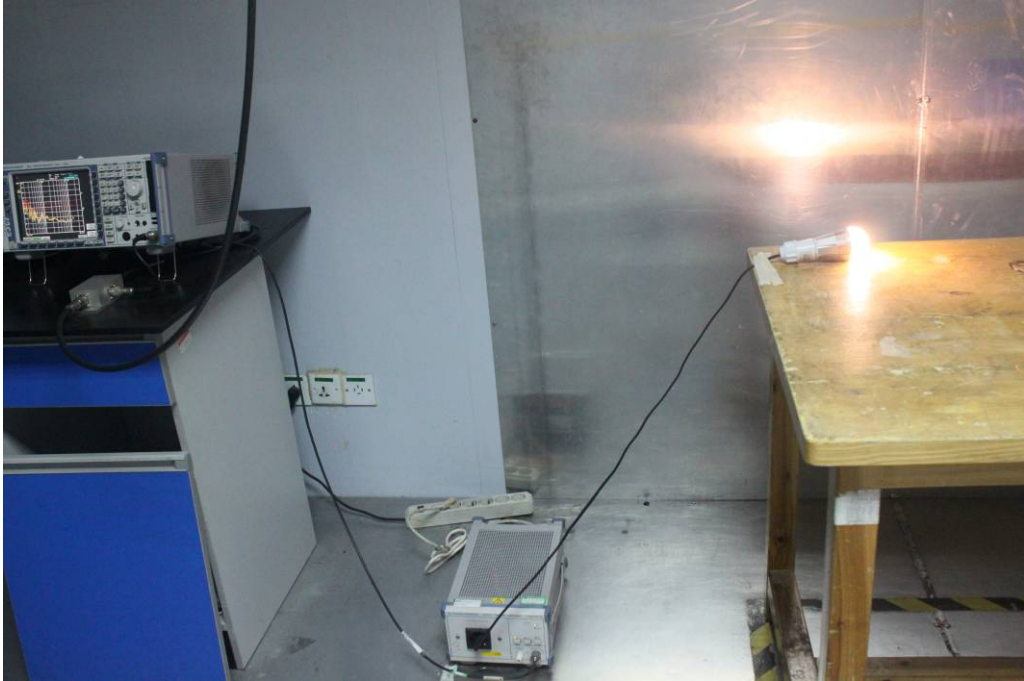
17.2 Photograph – Conducted Emission Test Setup
