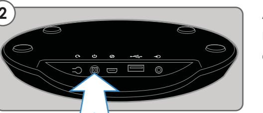
Attach the included power adapter to your receiver. Your receiver will automatically power on. The Wi-Fi light will blink quickly while the receiver is starting up.
