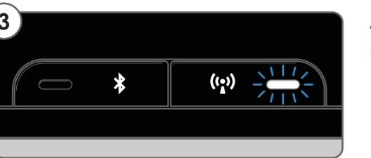
After 20 seconds the Wi-Fi light will begin to pulse slowly. The receiver is now ready to be set-up.
