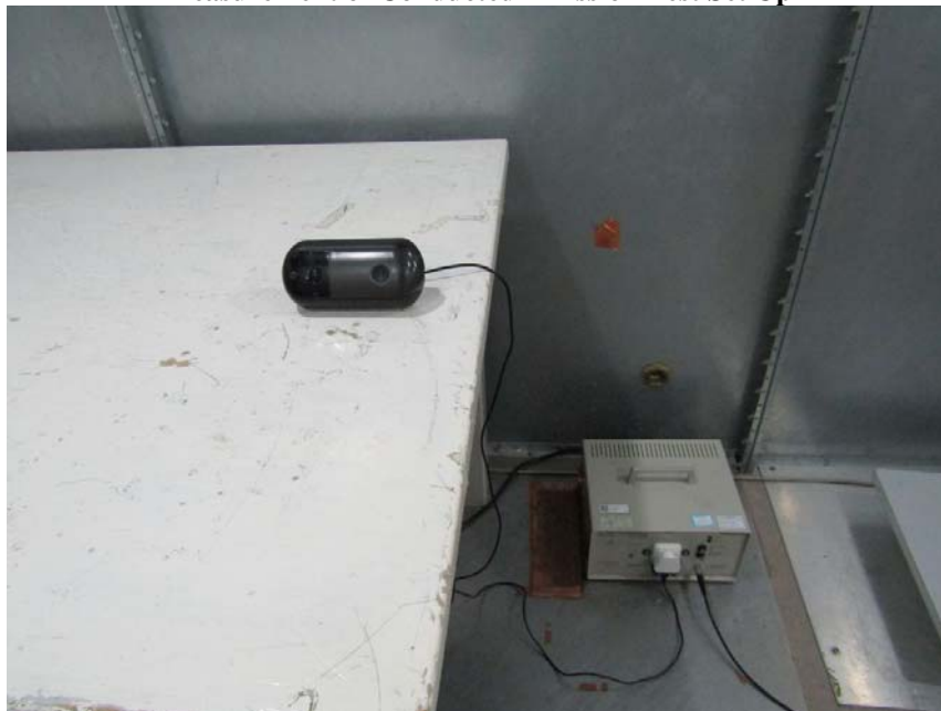
Measurement of Conducted Emission Test Set Up
