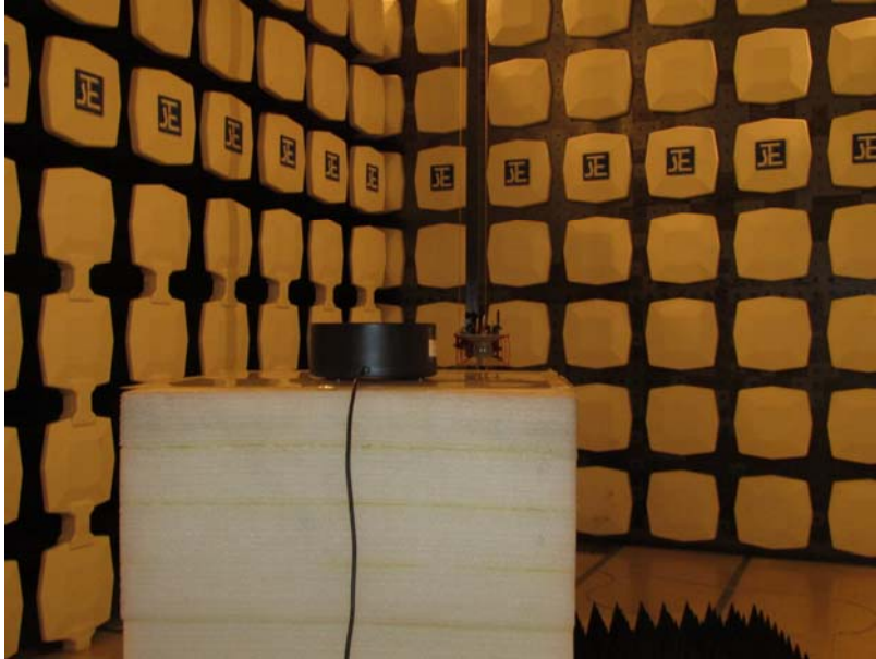
Measurement of Radiated Emission Test Set Up
