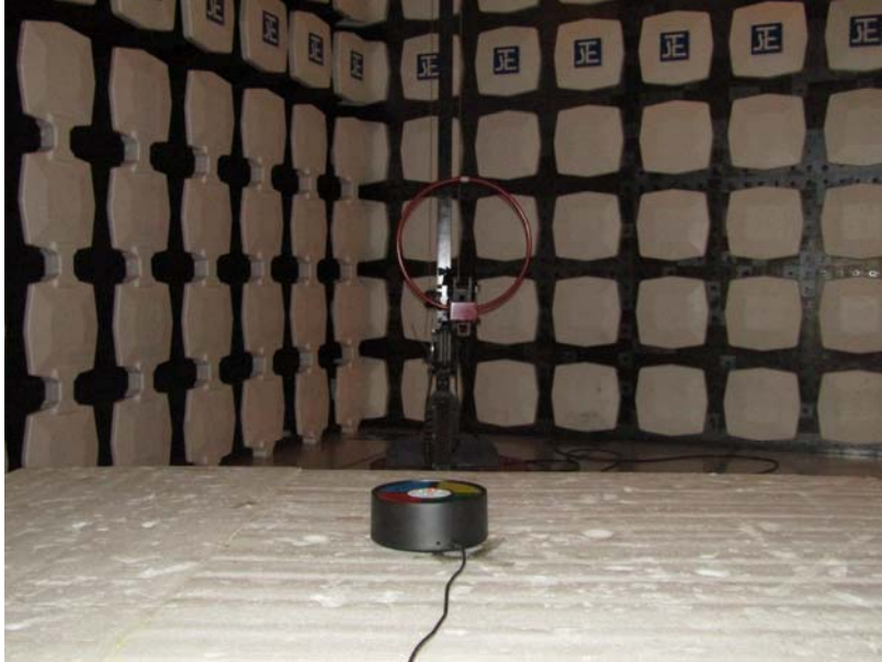
Measurement of Radiated Emission Test Set Up
