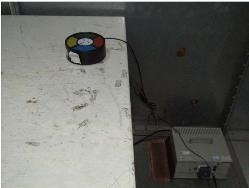
Measurement of Conducted Emission Test Set Up
