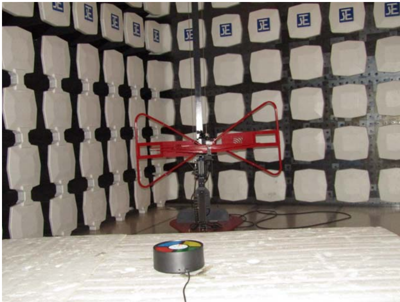
Measurement of Radiated Emission Test Set Up
