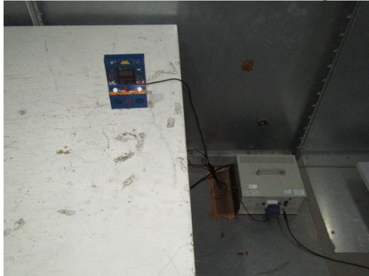
Measurement of conducted Emission Test Set Up
