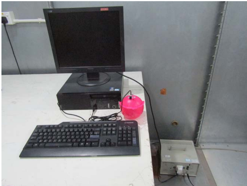
Measurement of Conducted Emission Test Set Up
