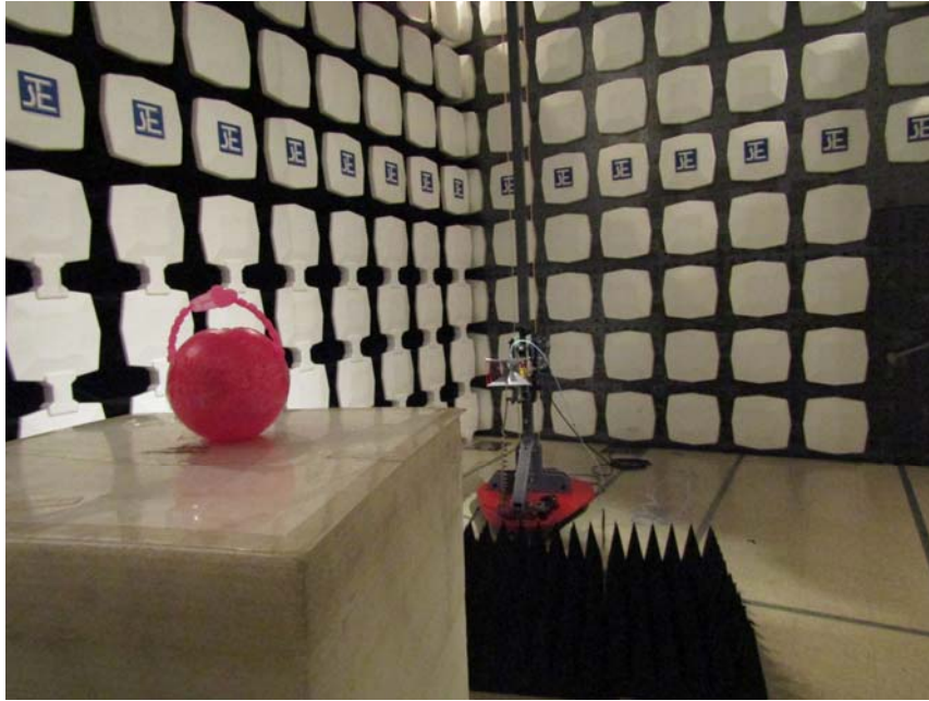
Measurement of Radiated Emission Test Set Up
