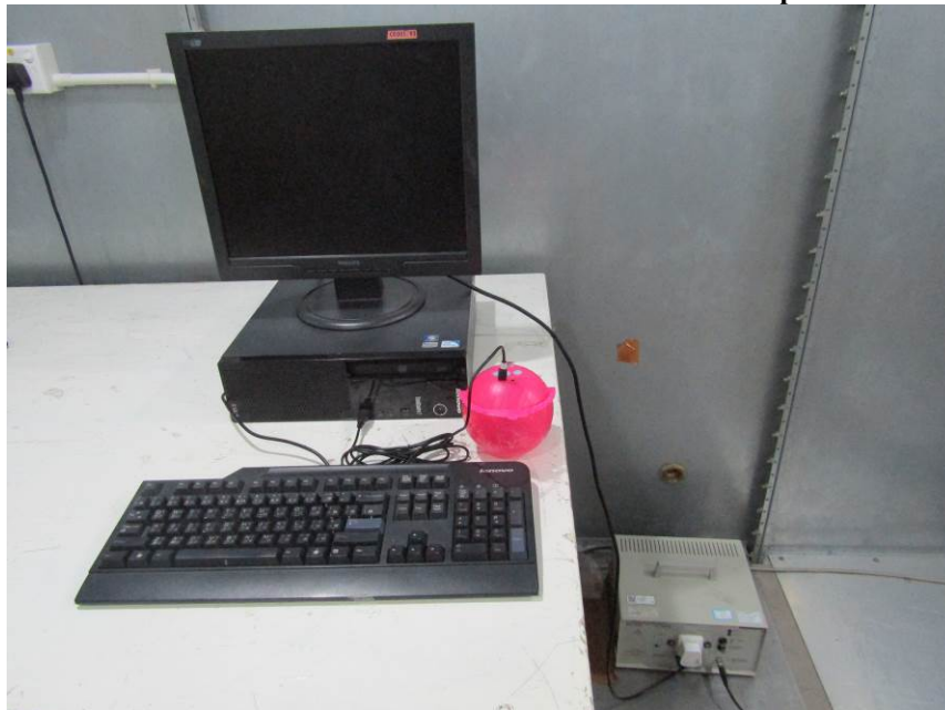
Measurement of Conducted Emission Test Set Up
