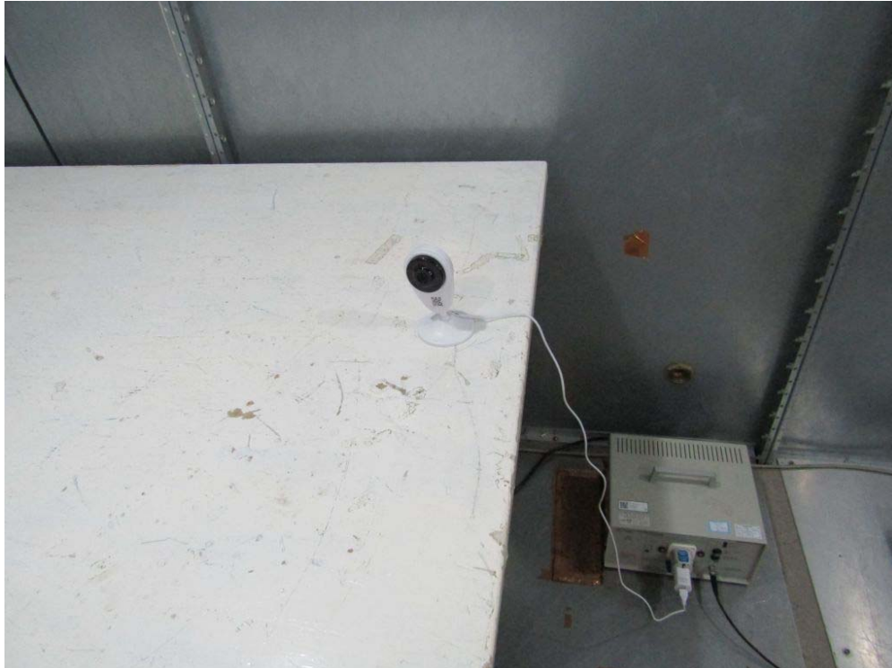
Measurement of Conducted Emission Test Set Up
