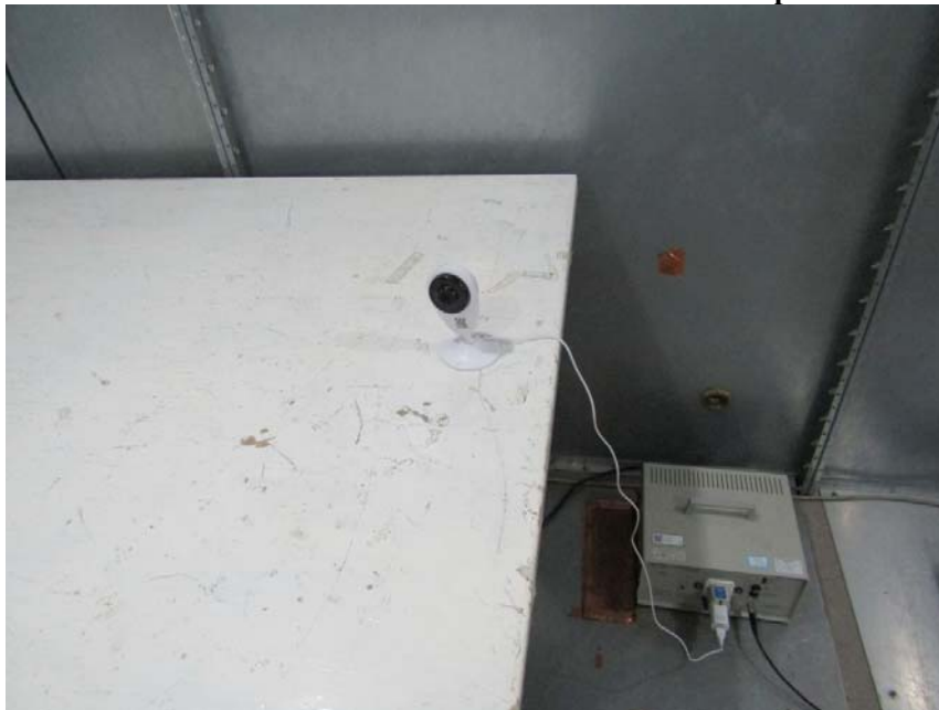
Measurement of Conducted Emission Test Set Up
