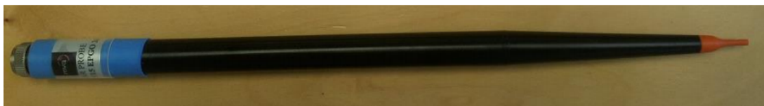
Figure 1 – MVG COMOSAR Dosimetric E field Dipole
