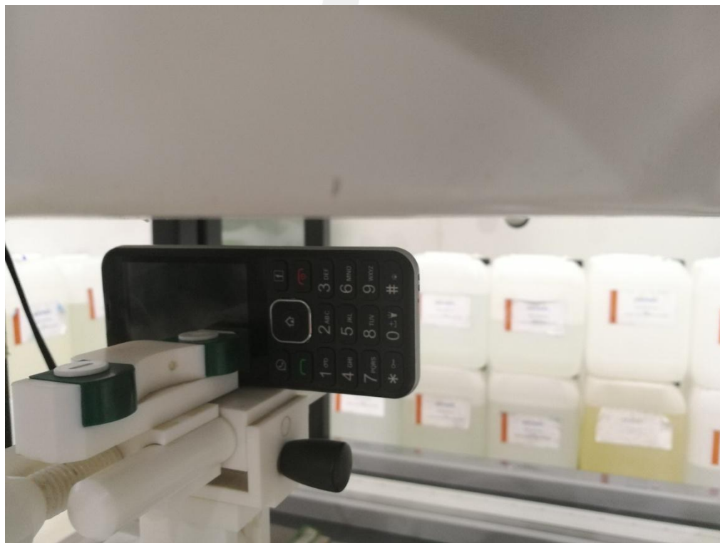
Body Right side(separation distance is 10mm)
