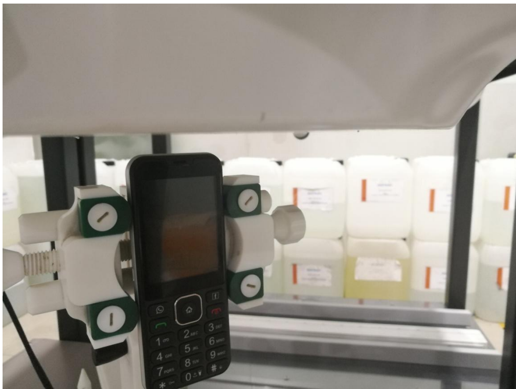
Body Top side(separation distance is 10mm)
