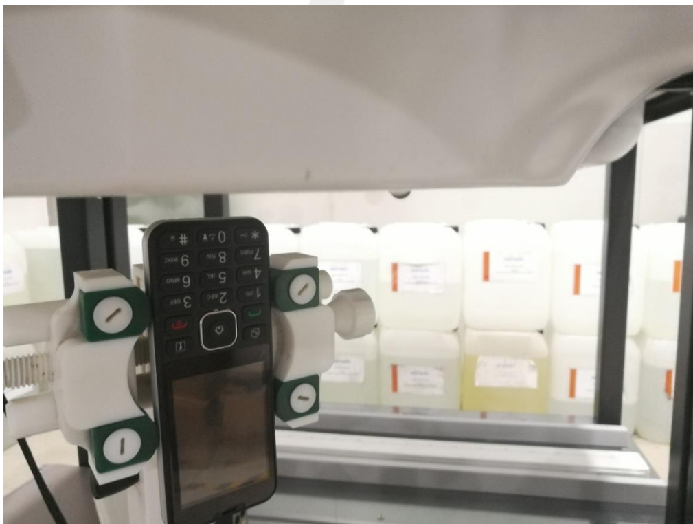
Body Bottom side(separation distance is 10mm)
