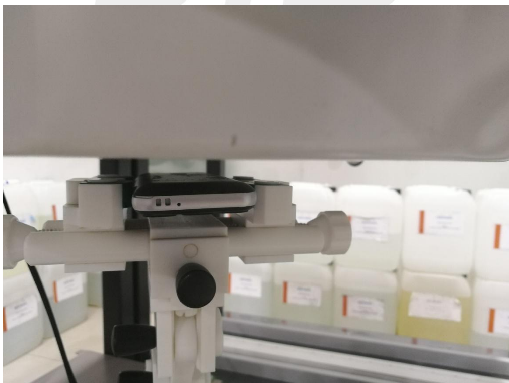
Body Back side(separation distance is 10mm)
