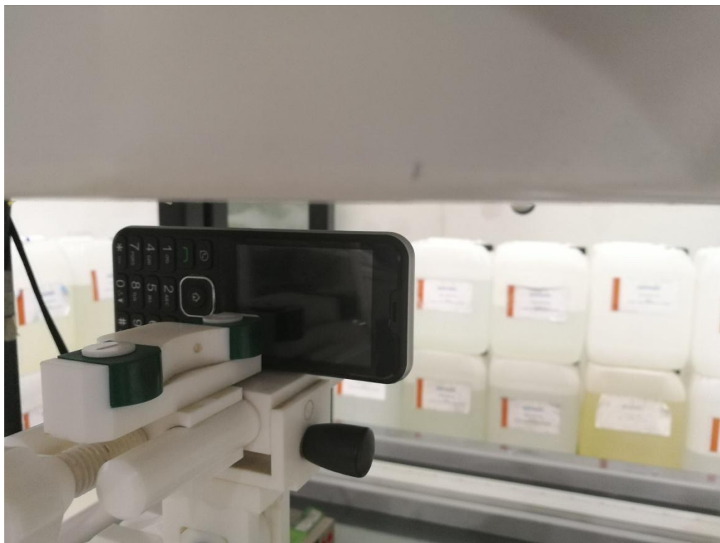
Body Left side(separation distance is 10mm)
