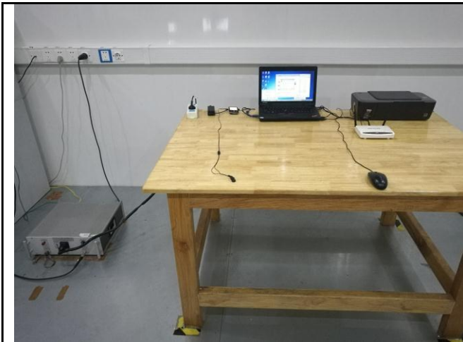
Conducted Emissions Test Setup – Front View
