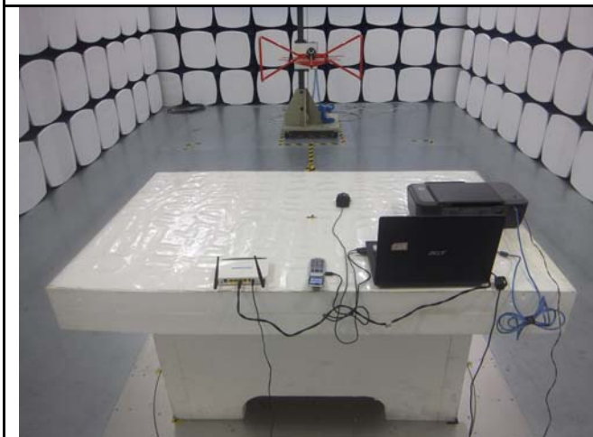
Radiated Emissions Test Setup Below 1GHz
