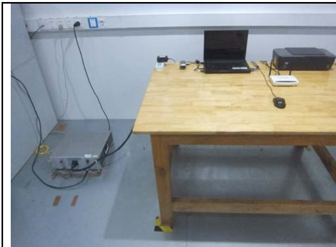
Conducted Emissions Test Setup – Front View
