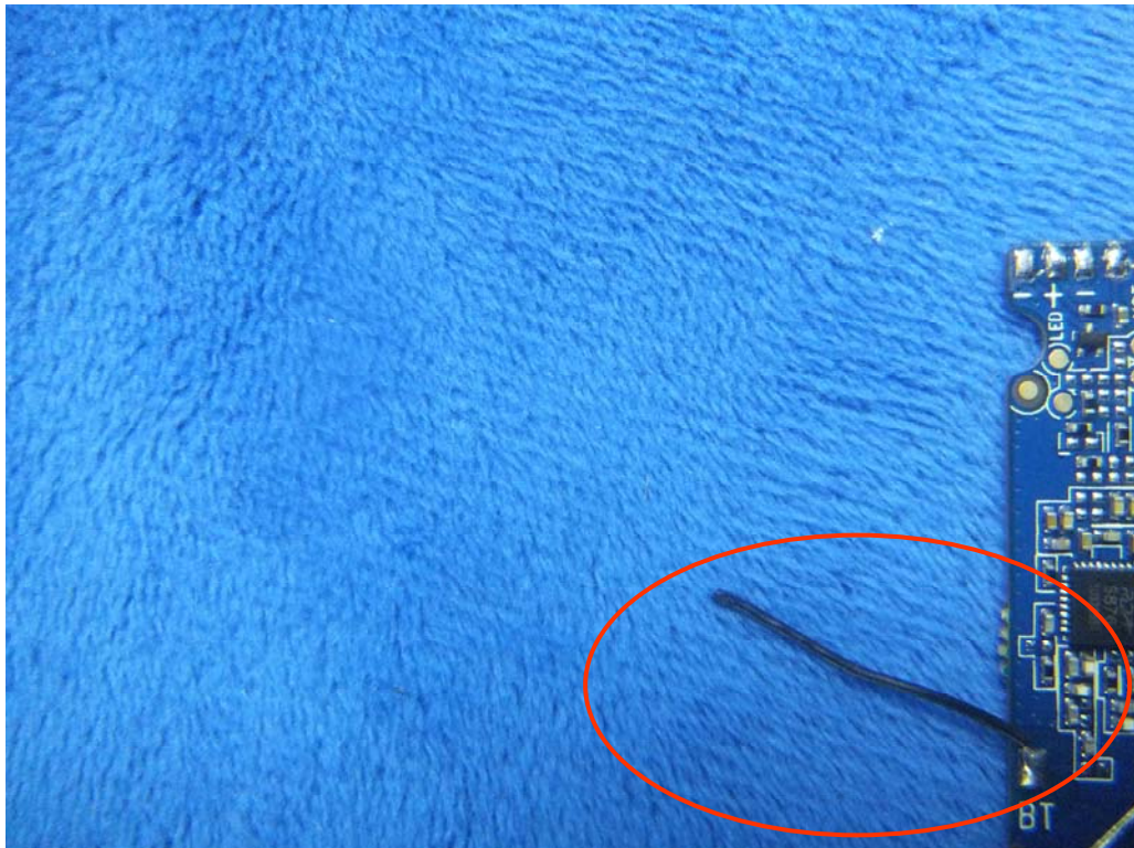
BT-FDD Antenna View
