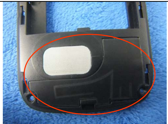
GSM/PCS Antenna View
