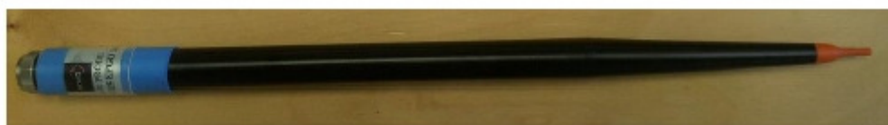
Figure 1 – MVG COMOSAR Dosimetric E field Dipole
