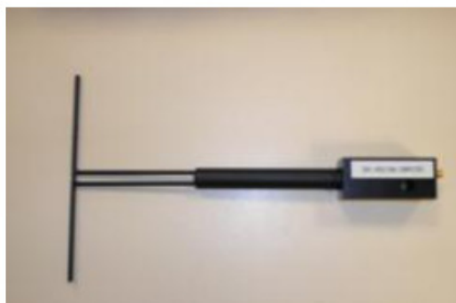
Figure 1 – Satimo COMOSAR Validation Dipole
