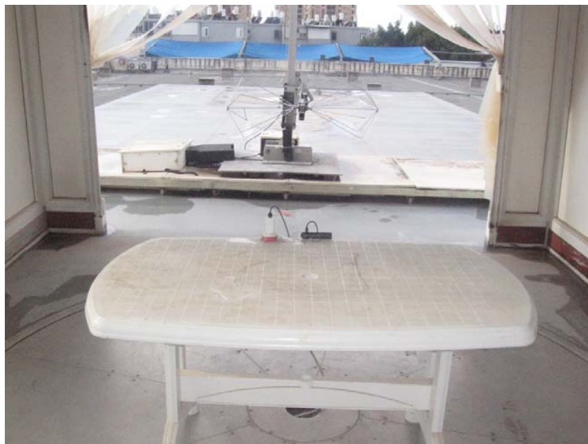
Figure 7. Radiated Emission Test, 30-200MHz
