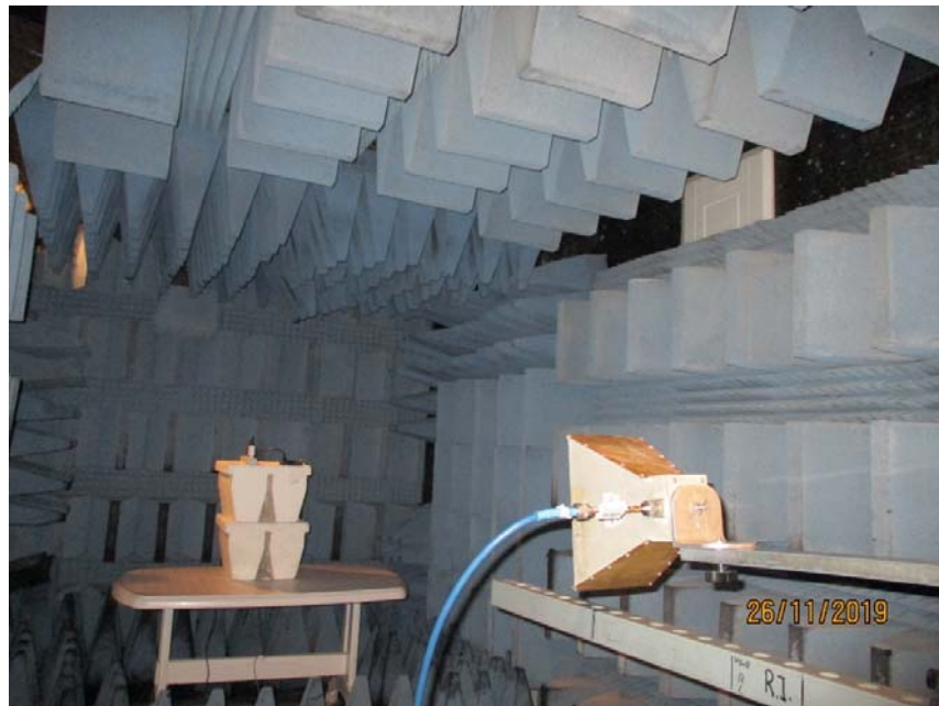
Figure 9. Radiated Emission Test, 1-18GHz
