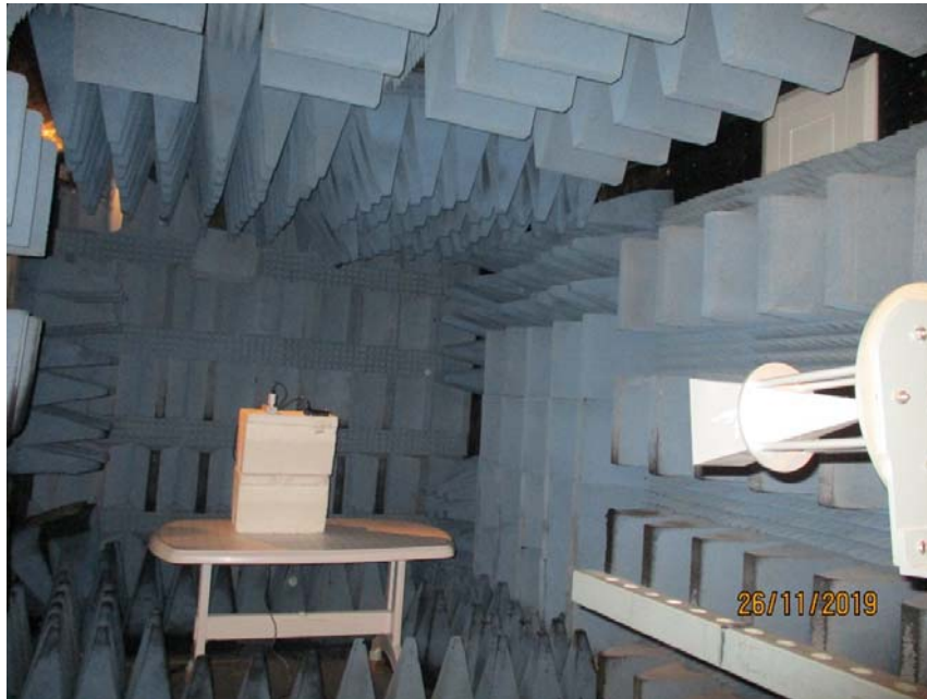
Figure 10. Radiated Emission Test, 18-26.5GHz
