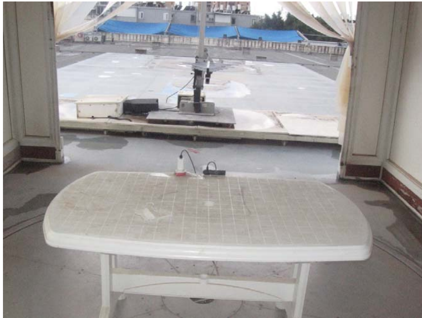
Figure 8. Radiated Emission Test, 200-1000MHz
