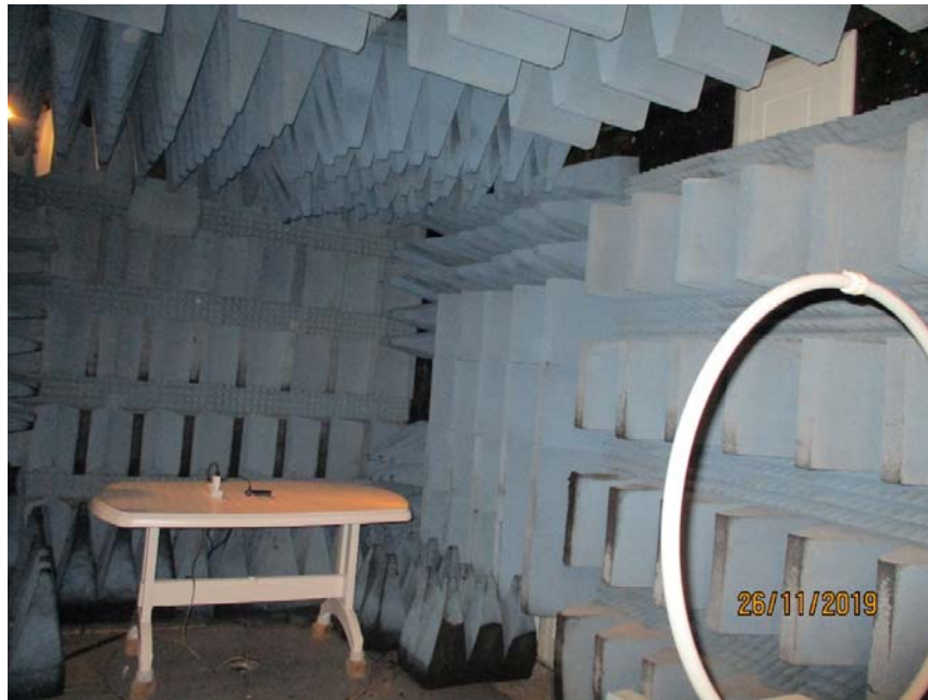
Figure 6. Radiated Emission Test, 0.009-30MHz
