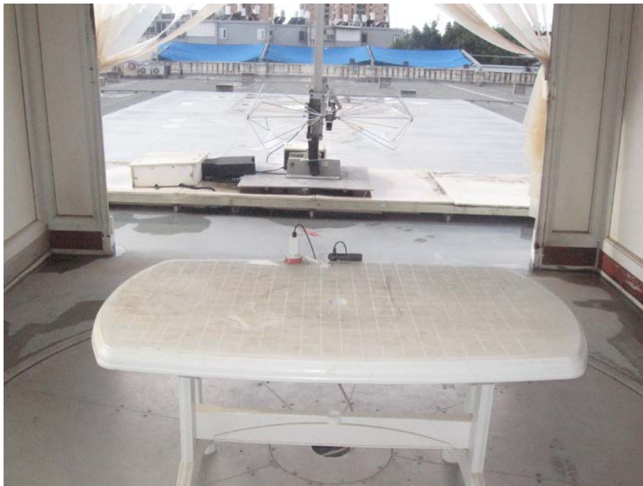
Figure 7. Radiated Emission Test, 30-200MHz
