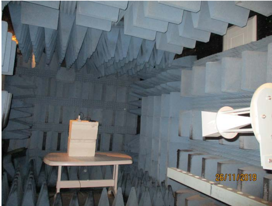
Figure 10. Radiated Emission Test, 18-25GHz
