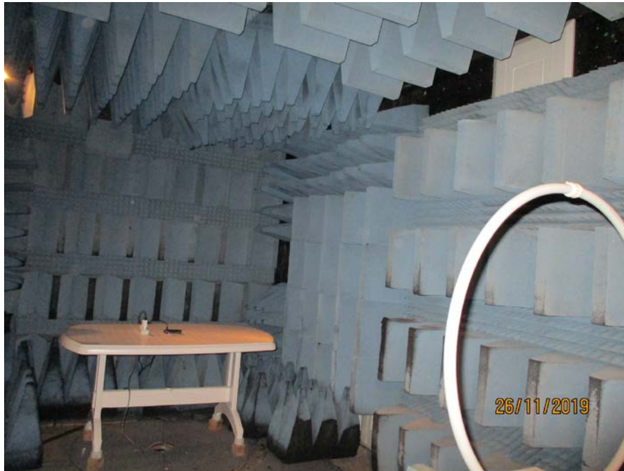
Figure 6. Radiated Emission Test, 0.009-30MHz
