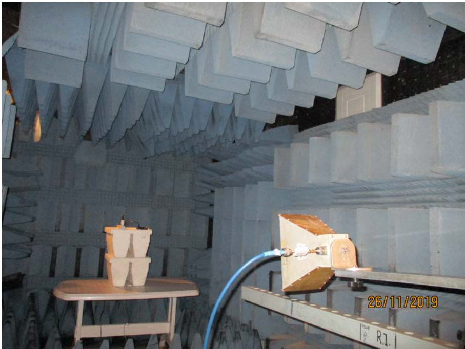
Figure 9. Radiated Emission Test, 1-18GHz
