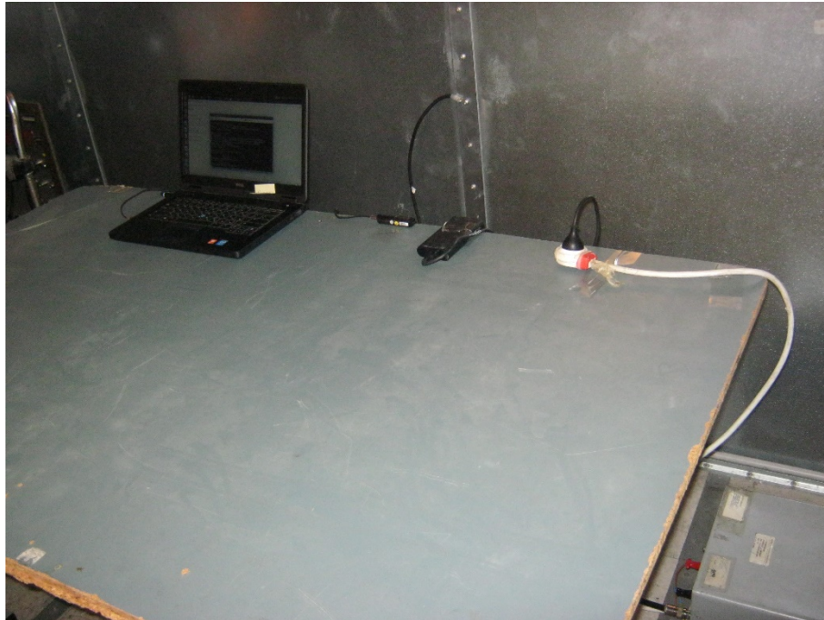
Figure 4. Conducted Emission from AC Line Test, AC/DC adapter via laptop charge mode
