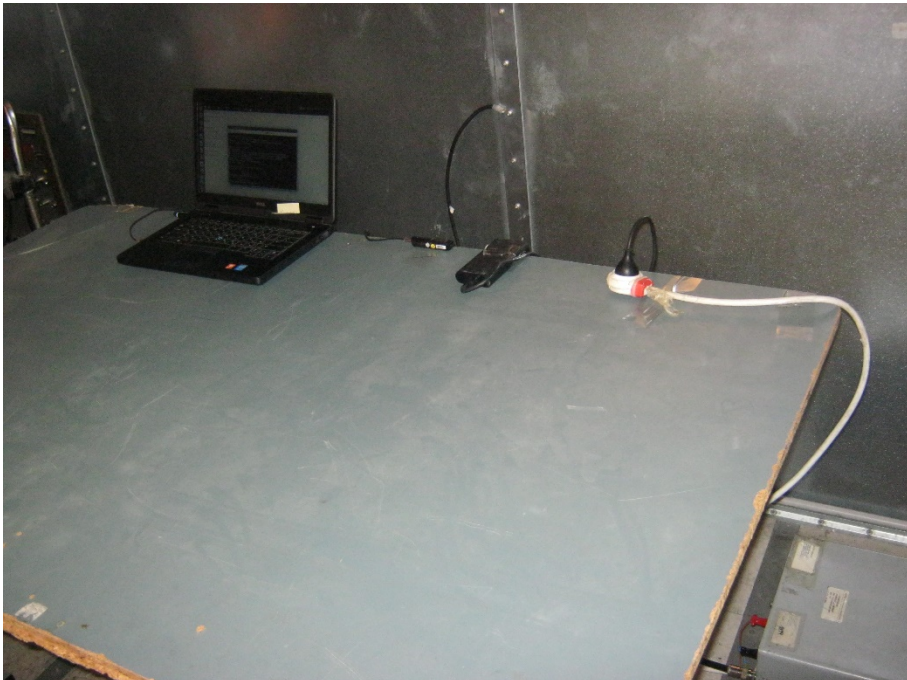
Conducted Emission from AC Line Test, AC/DC adapter via laptop charge mode
