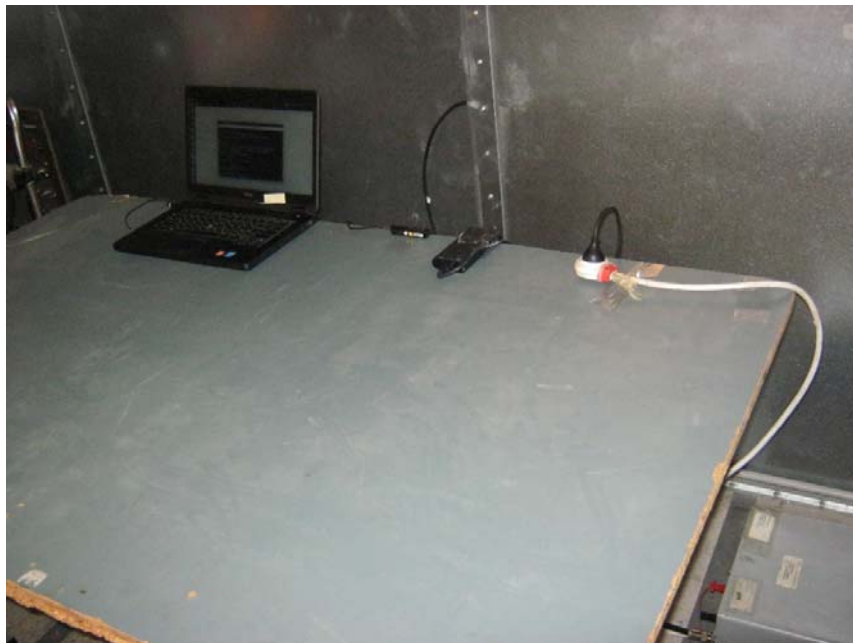
Figure 5. Conducted Emission from AC Line Test, AC/DC adapter via laptop charge mode
