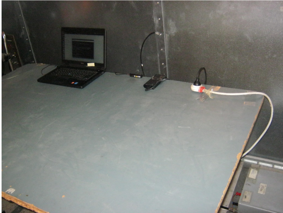
Figure 3. Conducted Emission from AC Line Test, AC/DC adapter via laptop charge mode
