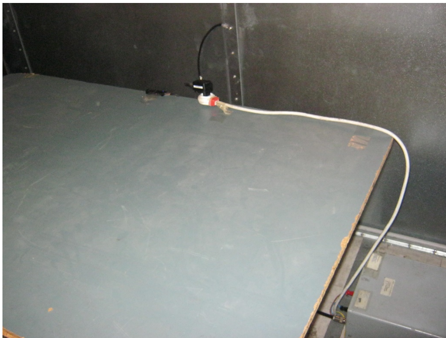
Figure 3. Conducted Emission from AC Line Test, AC/DC adapter via laptop charge mode
