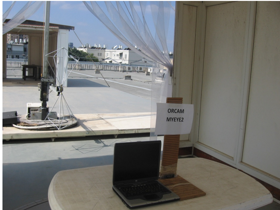
Figure 6. Radiated Emission Test - 30-200MHz
