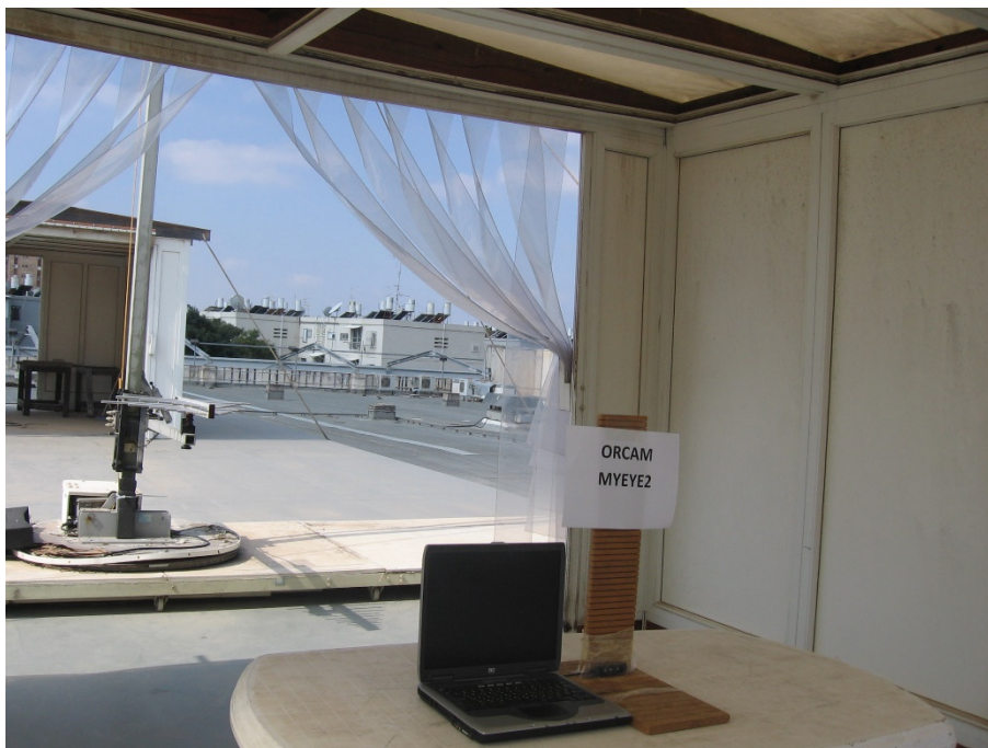
Figure 7. Radiated Emission Test - 200-1000MHz
