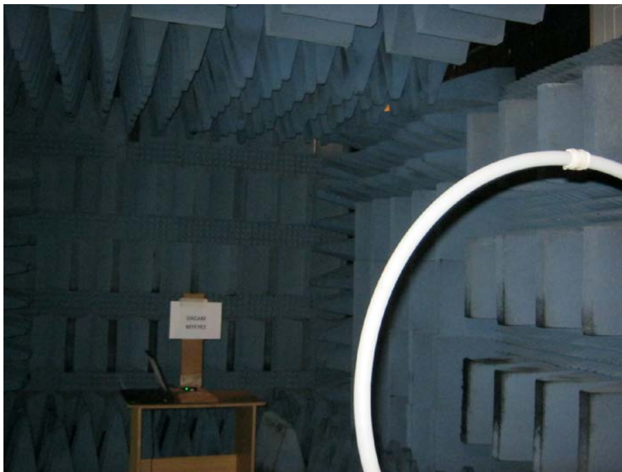
Figure 5. Radiated Emission Test - 0.009-30MHz
