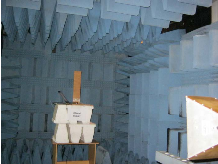
Figure 8. Radiated Emission Test- 1GHz-18GHz
