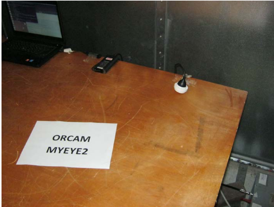
Figure 4. Conducted Emissions AC Line Test
