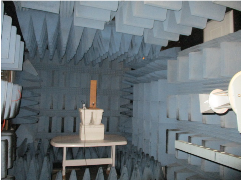
Figure 10. Radiated Emission Test, 18-26.5GHz
