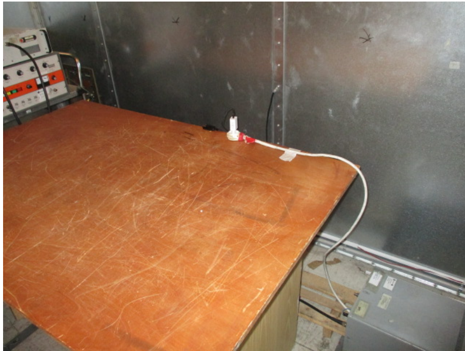
Figure 4. Conducted Emission Test from AC Line Test
