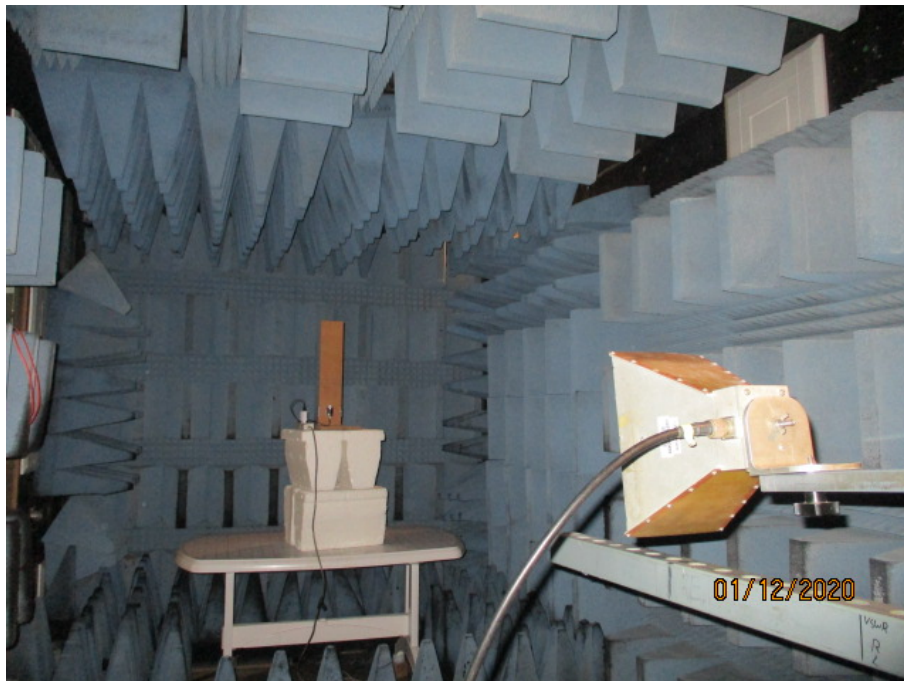
Figure 8. Radiated Emission Test, 200-1000MHz
