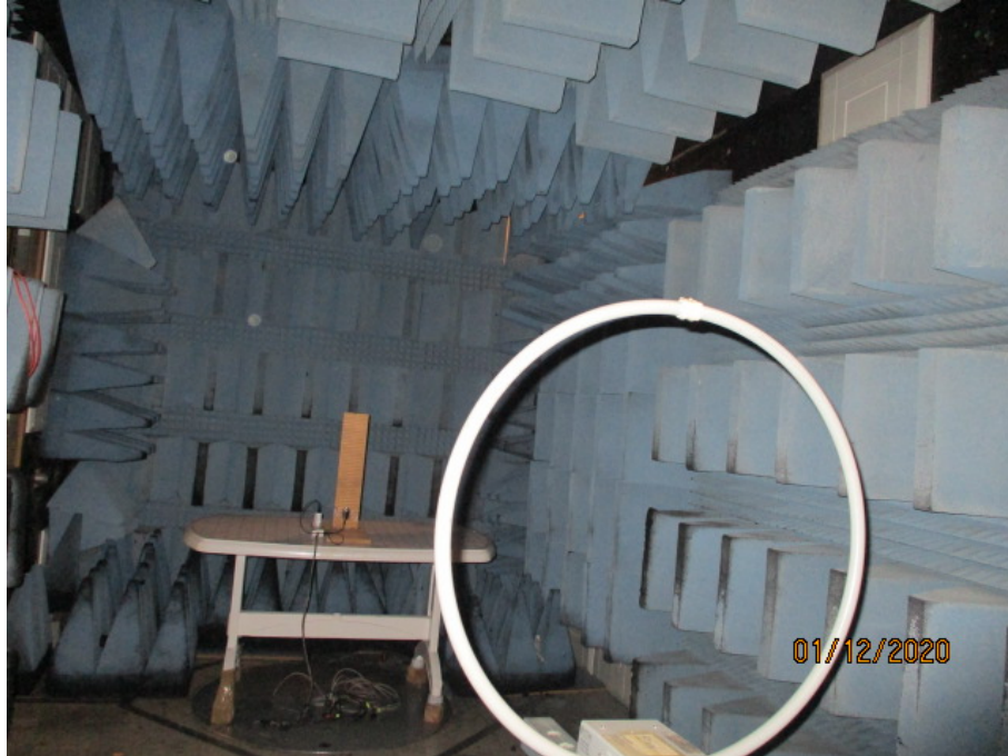
Figure 6. Radiated Emission Test, 0.009-30MHz
