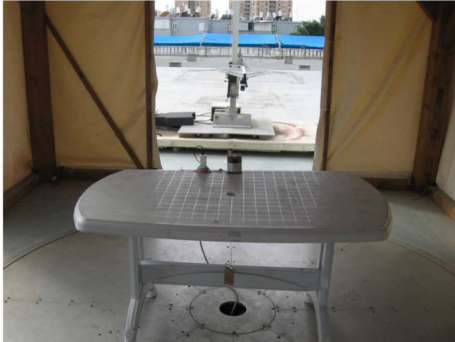
Figure 8. Radiated Emission Test, 200-1000MHz
