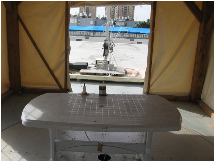
Figure 7. Radiated Emission Test, 30-200MHz
