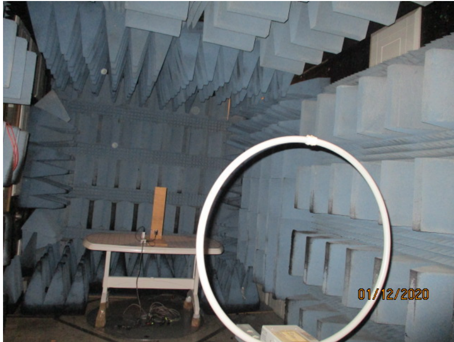
Figure 6. Radiated Emission Test, 0.009-30MHz
