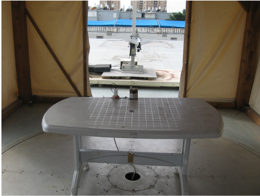
Figure 8. Radiated Emission Test, 200-1000MHz
