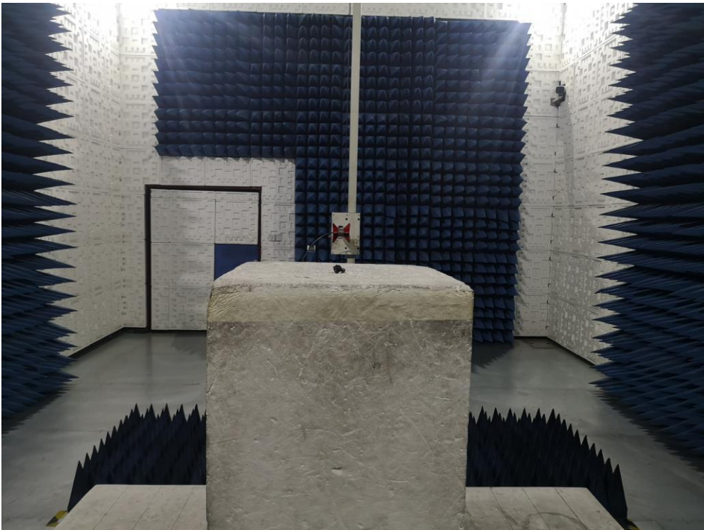
RADIATED EMISSION TEST SETUP ABOVE 1GHz
